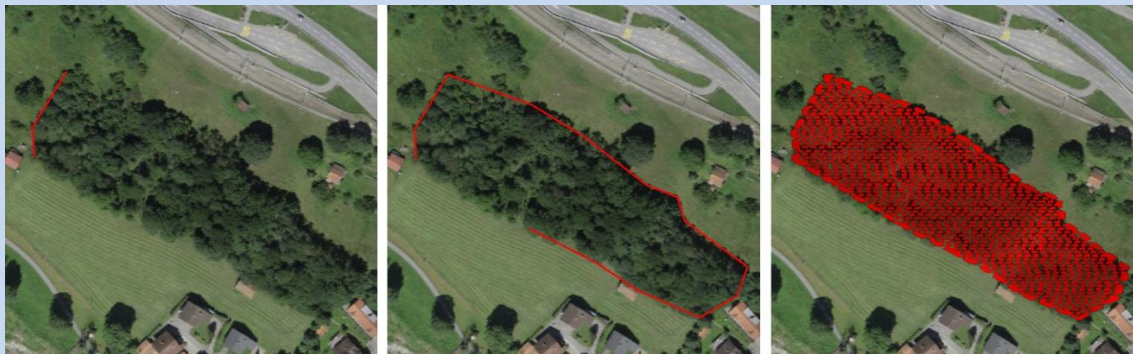
Figure 5-43: Project with emerging polygon shapefile (left, middle) and assigned dense forest (right).
