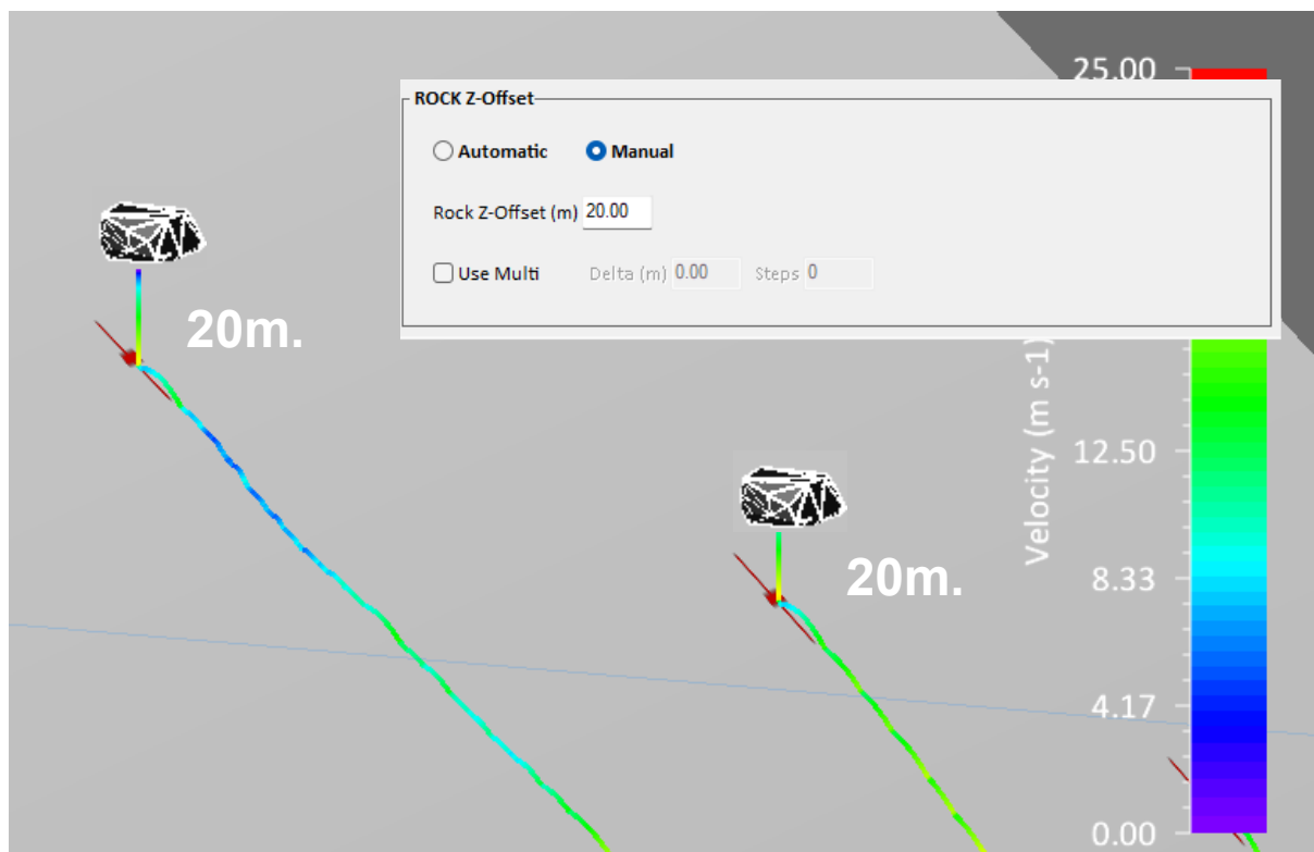
Figure 6-11: Definition of rock Z-offset in RAMMS::Rockfall. In automatic mode, the rock is positioned normal to the terrain surface to avoid initial intersection with the DEM. In manual mode, the rock is vertically offset from its center of mass, increasing its initial potential energy and influencing the impact energy and trajectory evolution.
